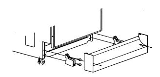
To lower the kickplate into position slide the kickplate vertically via the mounting slots to cover the dishwasher feet.
